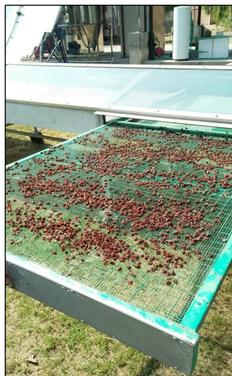
Figure 3: Grapes in solar tunnel dryer
