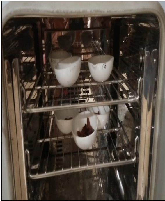
Figure 7: Moisture content determination of the raisin
