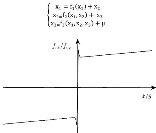
**Figure 3:** Friction relationship with the vehicle speed
