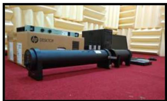
Figure 3: The Transmission Loss test using an Impedance Tube was carried out at the Building Science and Technology Laboratory, Department of Architecture, University of Hasanuddin. Foto: Asniawaty, 2021
