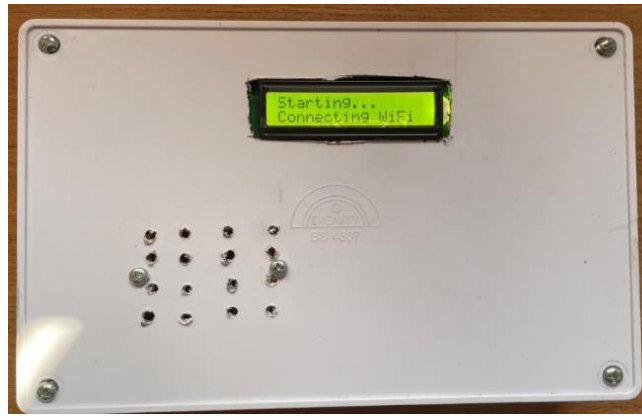
Plate 3.2: Packaging of the Hardware Circuit
